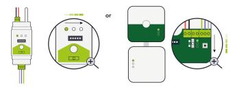
Set the RS485 bus settings on the gateway using the dip switches. These settings will automatically be used for all nodes in the network unless they have been manually set to local configuration ON. If autobaud is set to ON, the baud rate will be automatically discovered.
