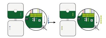
Return to the gateway and flip the 3-way switch to the "GATEWAY" (or Gateway position). This will lock and secure the network.
