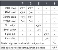
Install your W-Modbus node and connect it to your Modbus server device. Serial bus settings are inherited from the gateway unless local configuration is set to ON as described in Step 3.
