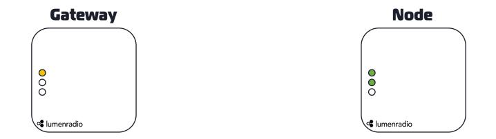
The Gateway will have a steady yellow LED on top and the node will have Top led as steady green. Second LED will be either steady green or steady red
